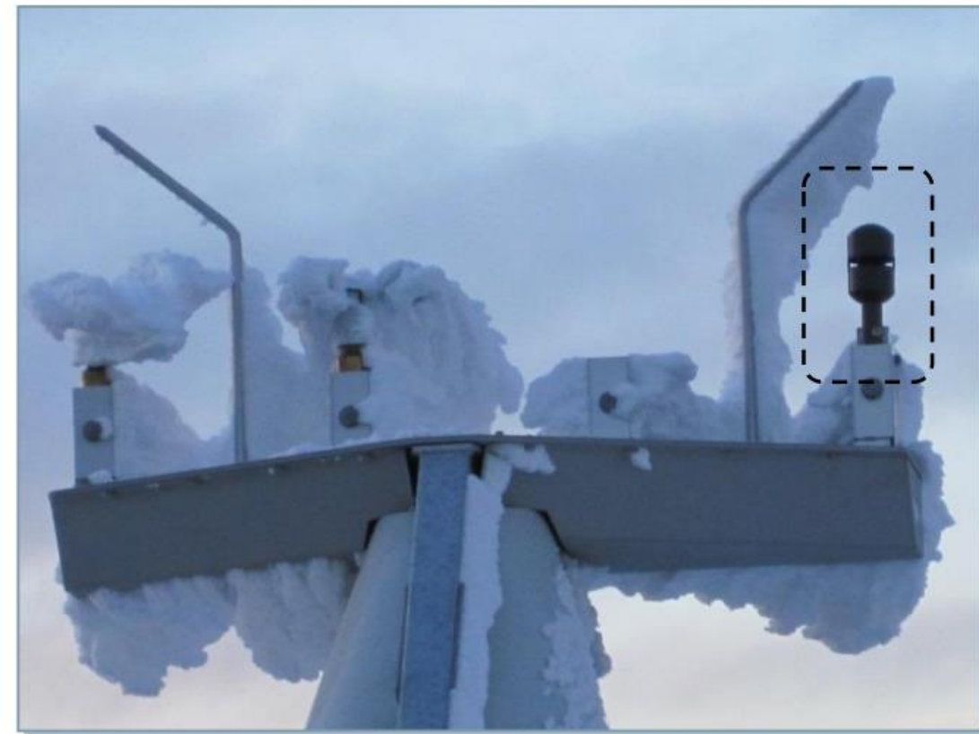
Ice-free sonic wind sensor with integrated heating (dotted line)
